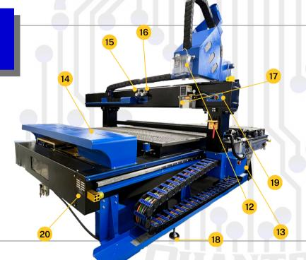
Mist Cooling Lubrication Tank 12
